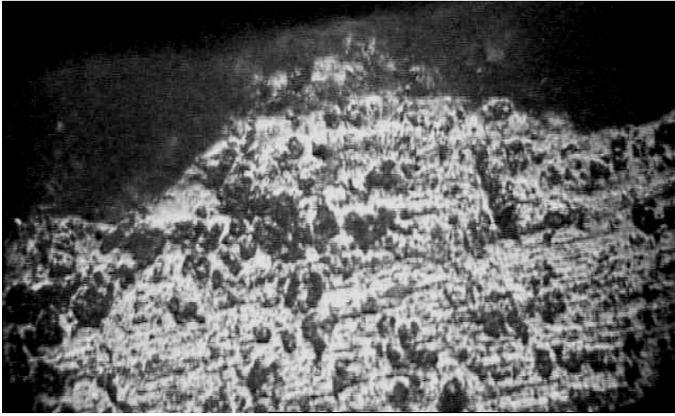
Fig. 1. Experimental chisel with edge-grinding traces running lengthwise ( \leftarrow ) and smooth, domed wood polish and striations normal ( \uparrow ) to the edge, used for approximately 3 h ( 100\times , width of the figure is approximately 650\ \mu\text{m} ).
