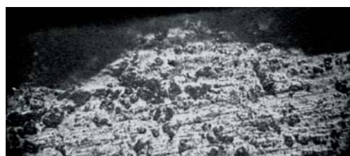
Fig. 8.1: Experimental chisel showing edge-grinding traces running lengthwise ( \leftarrow \text{⊗} \rightarrow ) and wood working traces oriented normal ( \bar{\downarrow} ) to the edge. (100x, width of figure is approx. 650 microns)
