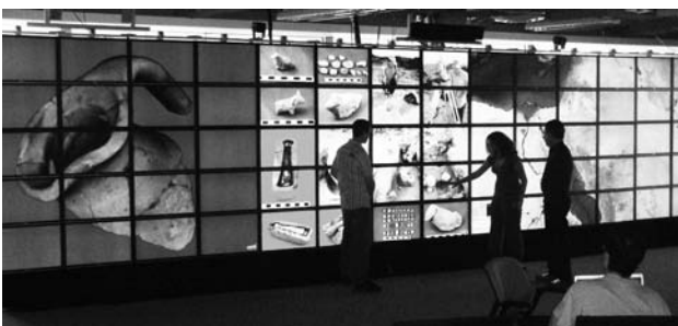
Figure 19. Interactive visualization and co-location of different artifacts from Jordan on HIPerSpace. The HIPerSpace is made with 72 ‘off-the-shelf’ Dell 3007WFP-HC, 30” displays or tiles (Photo: Falko Kuester, Calit2) .
